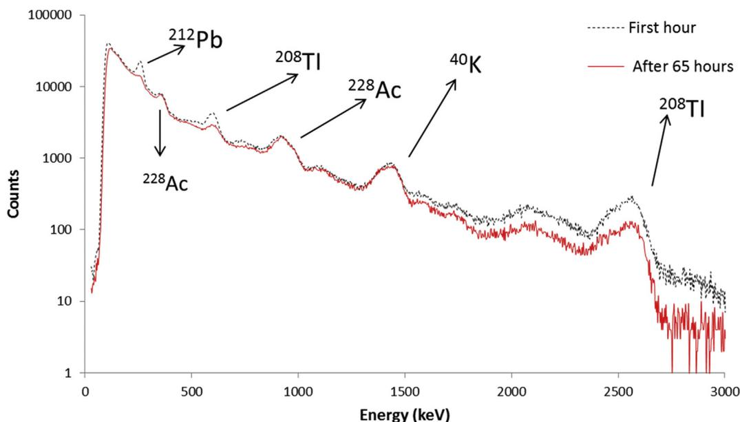
Fig. 3. Spectrum from the Solution during the first hour of measurement and after 65 h.
