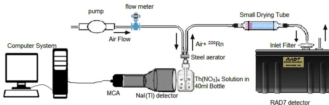
Fig. 1. The set-up used to measure the gamma rays from a solution while simultaneously bubbling air through the solution to provide a stream of air containing thoron that can be measured with the RAD7 as indicated.
