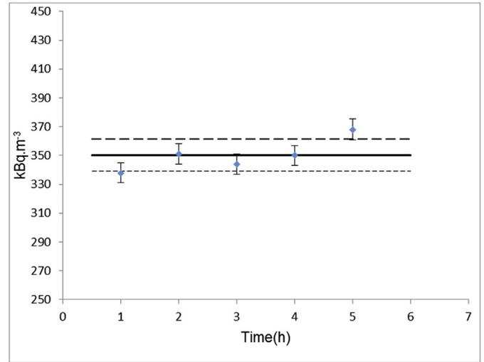
**Fig. 6.** The thoron concentration in the exit stream of the bubbler as obtained with the RAD7. The uncertainties are as given by the RAD7 based on statistical uncertainty. The mean value ( $350 \pm 11 \text{ kBq.m}^{-3}$ ) is indicated by the solid line whereas the dashed lines indicate the uncertainty. The measured values correspond well with the expected value as calculated from Eq. (2).
