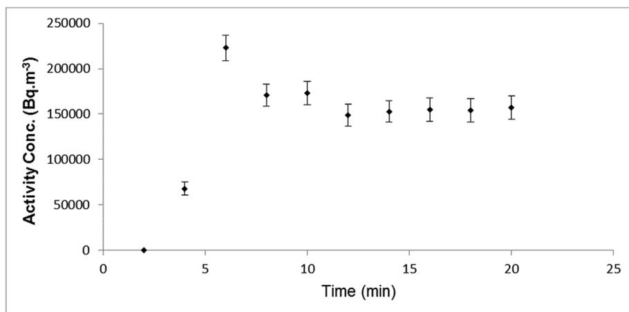
Fig. 7. Activity concentration as measured by the RAD7 during the initial few minutes of pumping for periods of 2 min. The pump was started at around  $t = 2$  min.
