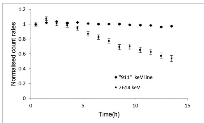
Fig. 4. Count rates in the “911” keV peak (diamonds) compared to the 2614 keV peak (squares).
